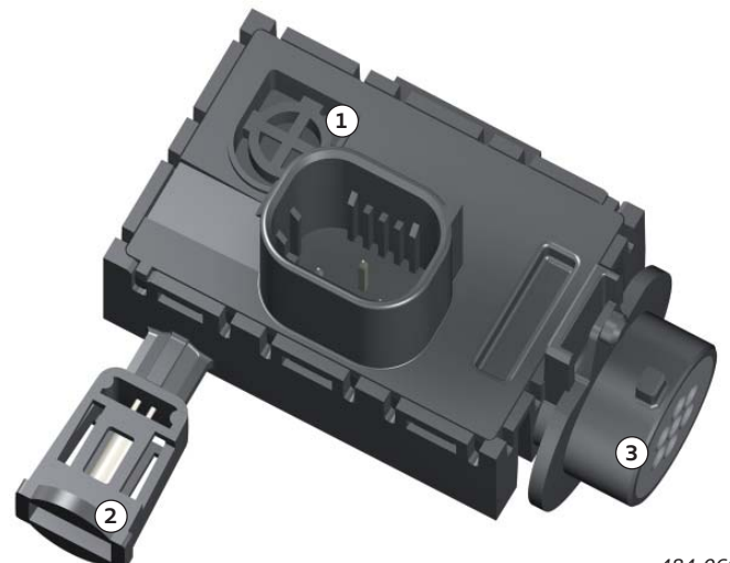
Air humidity sensor infresh air duct G657 with air quality sensor G238 in the four zone air conditioning system
