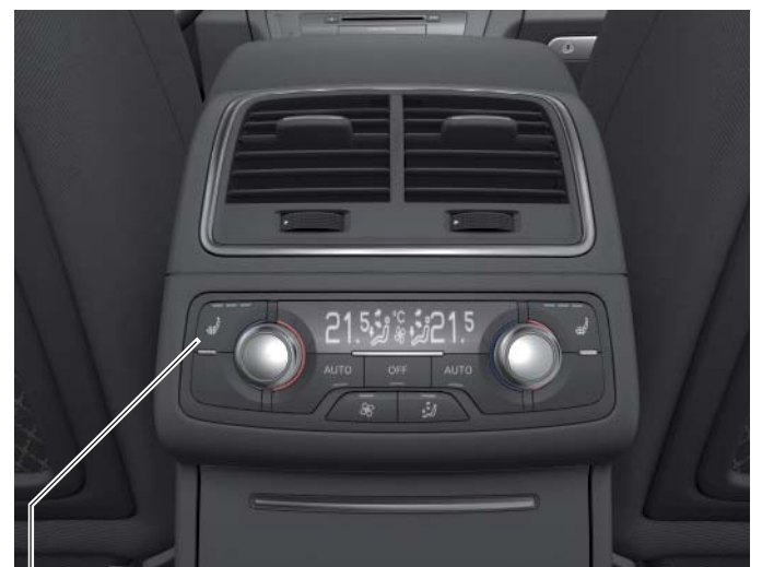
Rear seat heater with three settings
