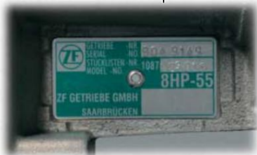
The type plate is located under the Flange shaft (visible from below)
